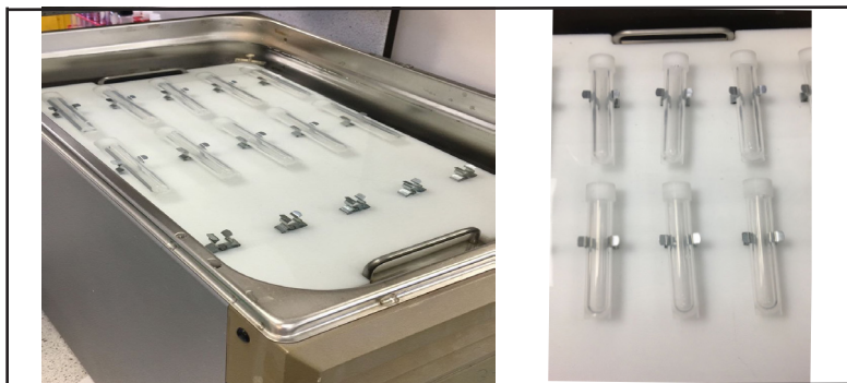
Figure 1. Attachment of 13 mL polypropylene tubes to a polypropylene tube-holder in a Grant OLS 200 water bath. Process Systems, Biopharma House, Winchester, UK.
