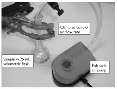
Figure 2. Arrangement for the oxidation of D-glucose by glucose oxidase plus catalase in the presence of a stream of air.
