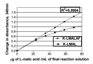
Figure 1. Calibration curve showing extended linearity of K-LMALAF as compared to K-LMAL. The reactions used to generate these calibration curves were performed at 25°C for 3 min, using a 4.6 mm path-length cuvette.
