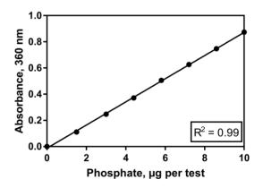
Figure 2. Linearity of the phosphate assay
