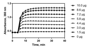
Figure 3. Increase in absorbance at 360 nm on incubation of 0-10 µg of phosphate per test
